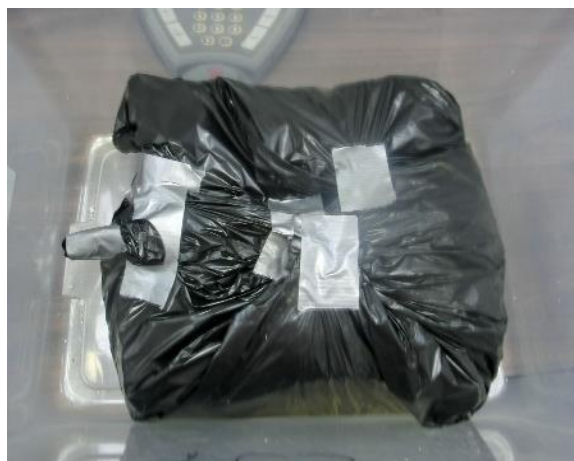
Figure 20: Wrapped sample being saturated
