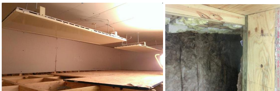
Figure 16: Thermally controlled top portion (Left) lower interior chamber open to ambient Temperature (Right).
