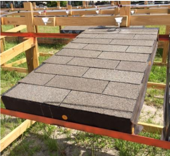
Figure 32: Membrane installed on all edges to prevent uncontrolled moisture travel
