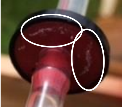
Figure 39: Whitish deposits observed on drippers after 6-weeks in use.
